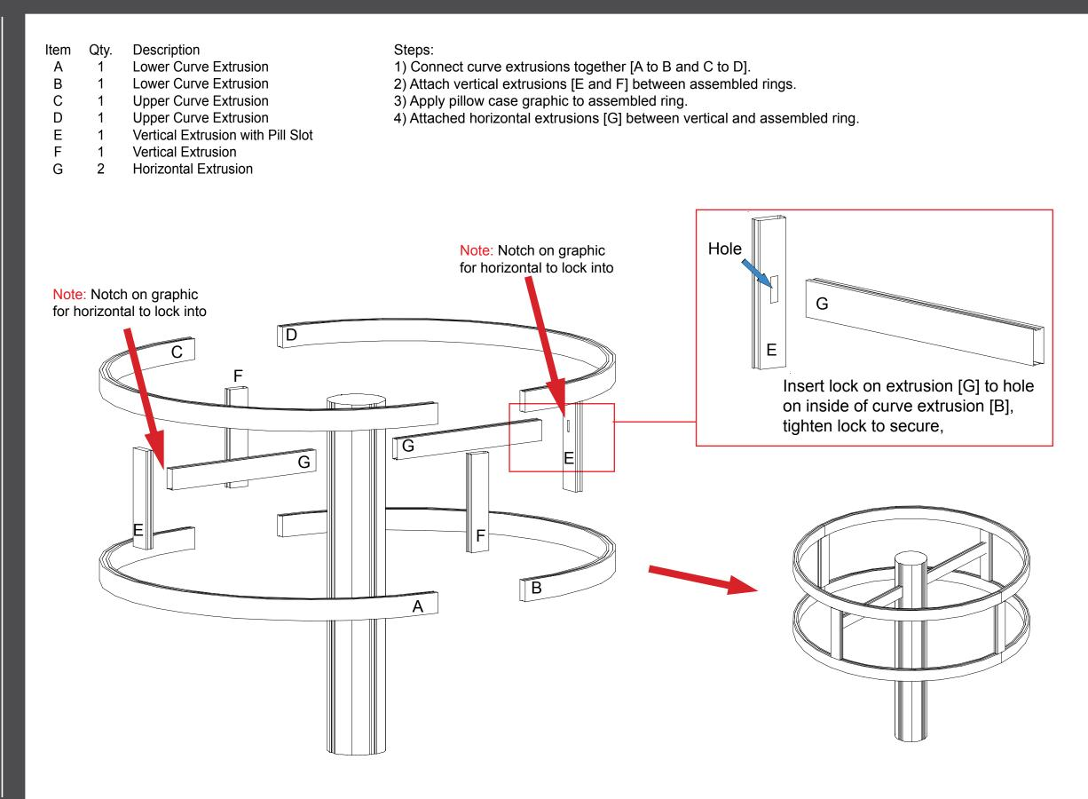
WHEN DISASSEMBLING ALUMINUM EXTRUSION, TIGHTEN ALL SETSCREWS AND LOCKS TO PREVENT LOSS DURING SHIPPING
